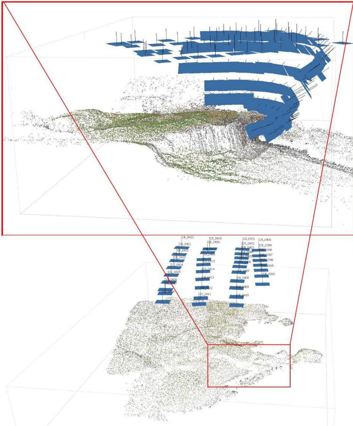
Figure 9: Point clouds and camera positions/orientations from the first survey (top) and the second survey (bottom)
