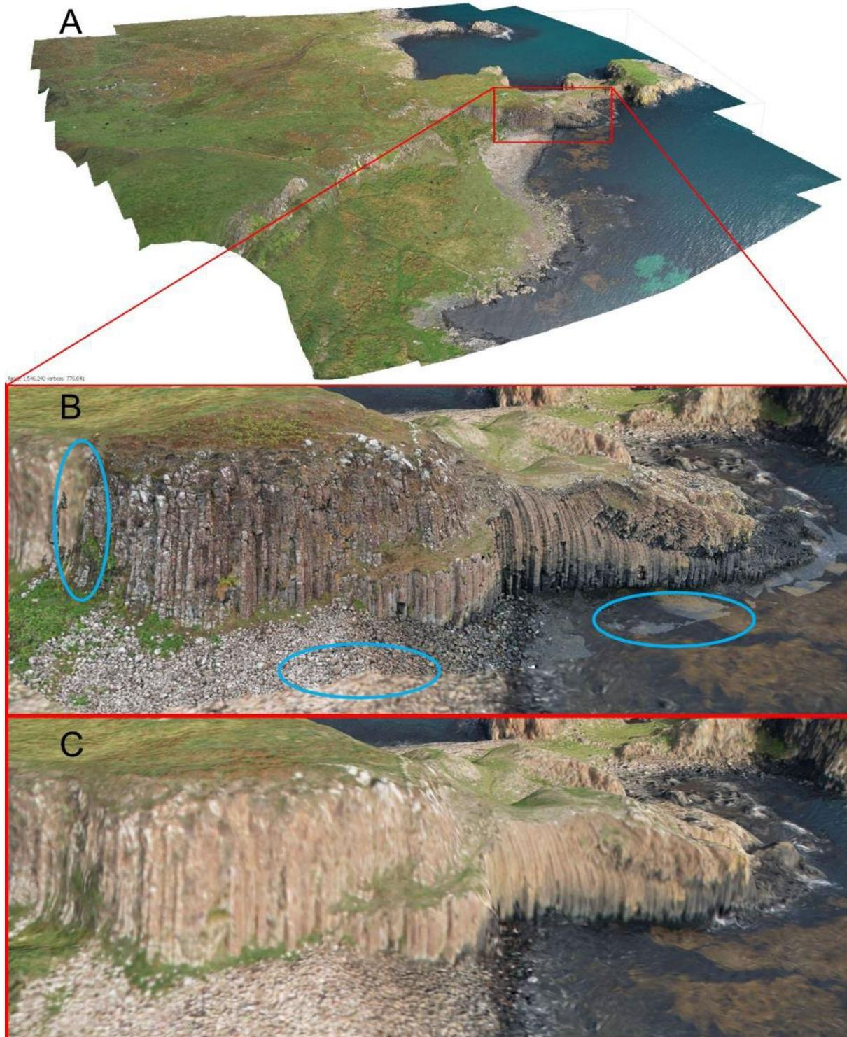
Figure 13: The overall merged model (A), and zoom in of the detailed section from survey 1 with blue ellipses highlighting where the two model resolutions meet (B) and the same area as B but from the low resolution model from survey 2 (C).
