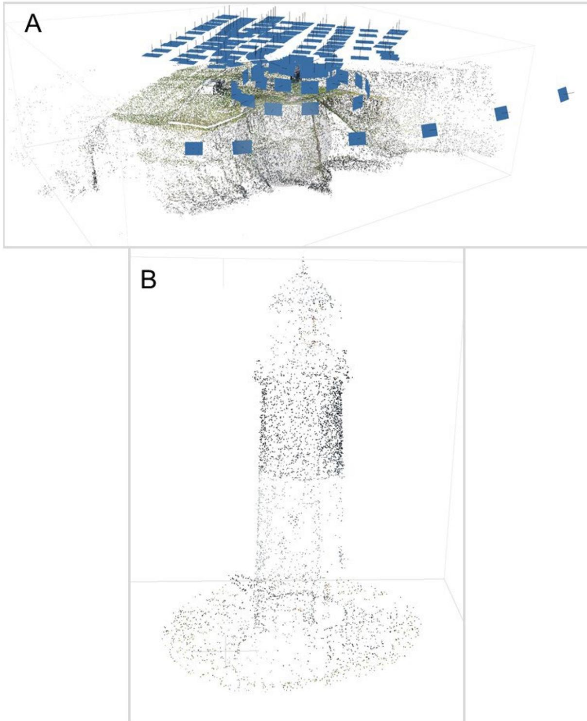
Figure 14: Survey 1 (A) showing the sparse point cloud and camera positions and the sparse point cloud from survey 2 (B)
