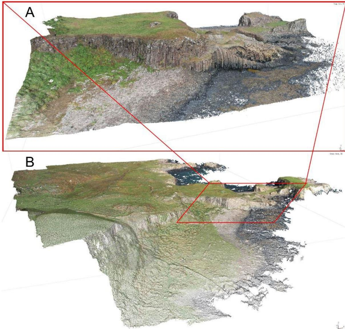
Figure 10: Dense point cloud from survey 1 (A) and survey 2 (B)
