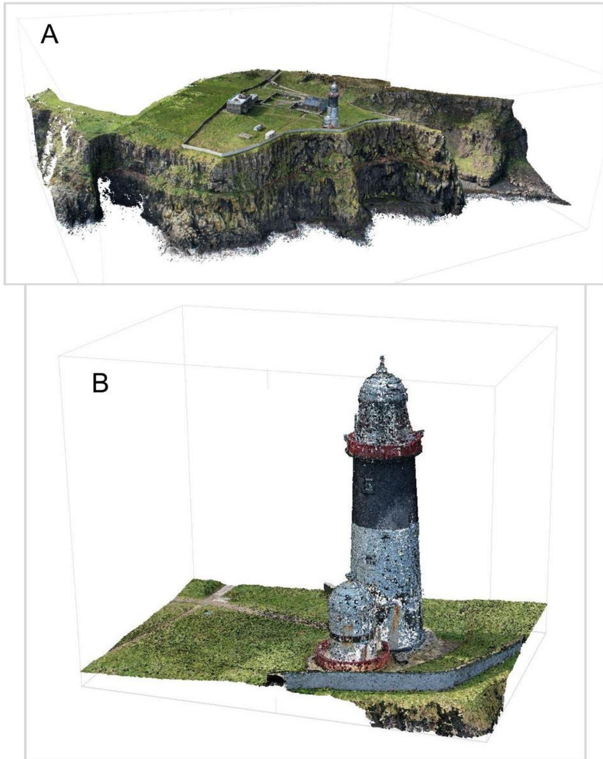
Figure 15: The dense point clouds from survey 1 (A) and survey 2 (B)
