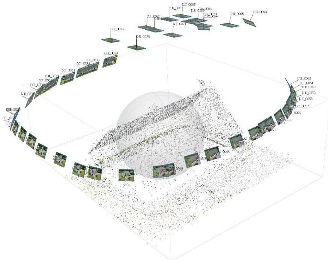
Figure 6: Sparse point cloud of the house with camera positions and orientations
