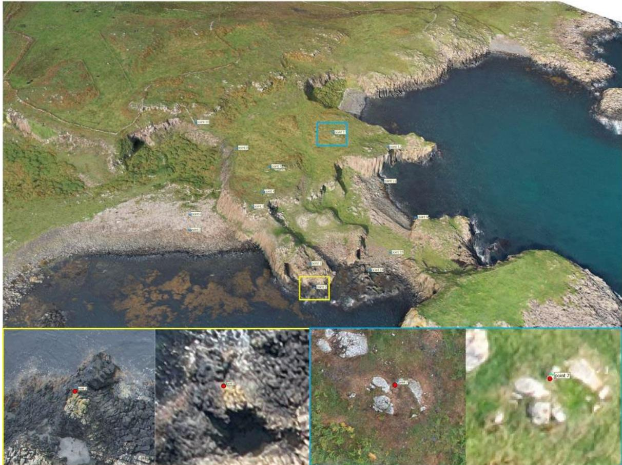
Figure 12: 15 markers distributed across the overlapping area of each dataset (top) and close up examples from photos in each data set for two of the markers (bottom).
