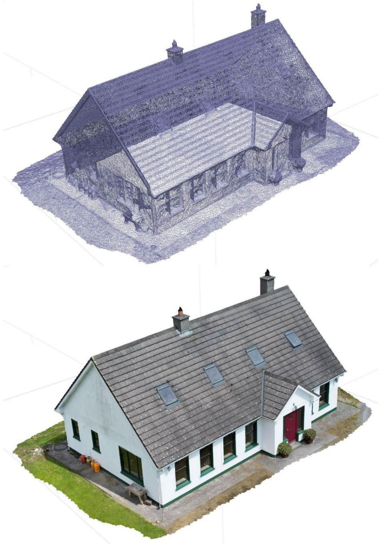
Figure 8: Mesh model (top) and textured model (bottom) of the house
