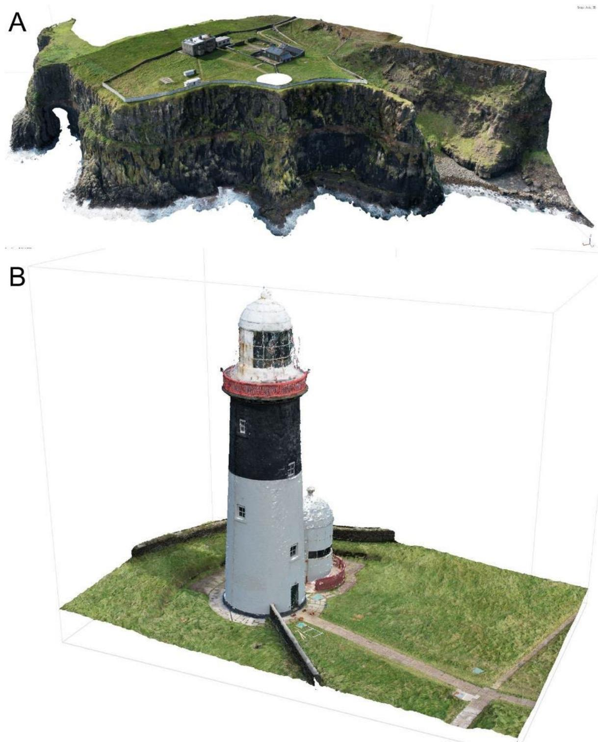
Figure 17: Model from survey 1 with the lighthouse cut out (A) and model from the detailed lighthouse survey 2 (B)
